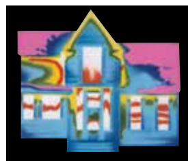
Before siding insulation. Energy transfers through the studs and siding.
