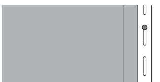
Fasten at the top uppermost unobstructed nail slot on the panel towards the top of the wall. DO NOT fasten through nailing flanges or any other accessories.
