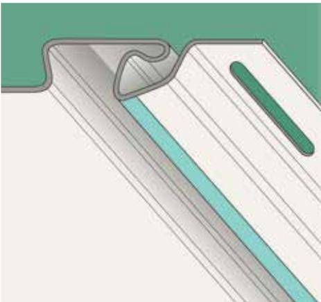
Charter Oak soffit is one of the most rigid soffit products on the market. Its superior rigidity is the result of Alside's exclusive TriBeam system. The result is a panel that's not only stiffer than competitive panels, but also lighter and easier to install.
