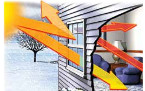
Winter Energy Savings: Low-E insulating glass helps reduce heat loss by reflecting warmth back into your home.
