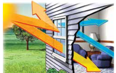
Summer Energy Savings: Low-E helps block unwanted solar heat penetration to help conserve air-conditioning use.
