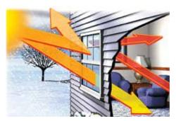
**Winter Energy Savings:** Low-E insulating glass helps reduce heat loss by reflecting warmth back into your home.
