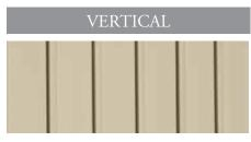
**Board & Batten** Faithful to its original design from centuries ago, this vertical panel features a 5-1/2" board face and a 1-1/2" batten strip that projects 1/2" above the board surface.
