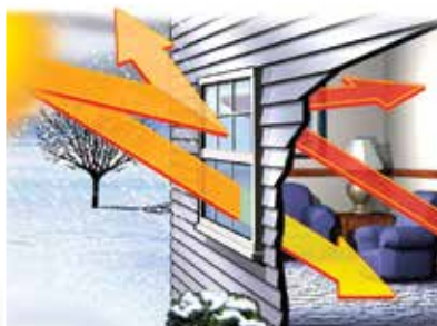
Low-E glass takes on a new duty in winter months by slowing indoor heat from escaping.
