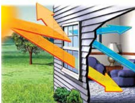
In summer months, Low-E glass helps block unwanted solar heat gain.
