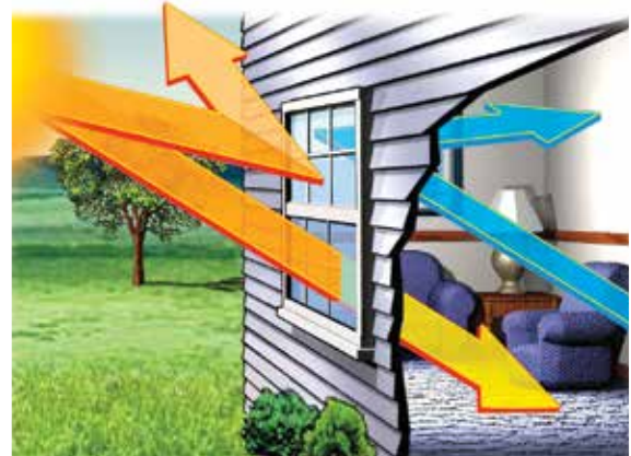
Low-E glass filters long-wave radiation from the sun. This helps reduce solar heat gain from the summer sun, helping to keep your home cooler.
