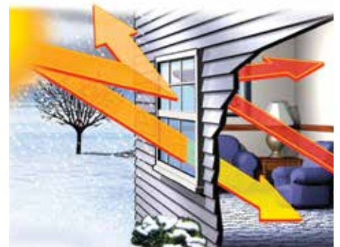
In winter months, Low-E reduces heat loss by reflecting warm air back into your home.
