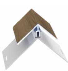
UNIVERSAL 2PC OUTSIDE CORNER AVAILABLE IN 2" & 3.5" (ALL ALUMINUM OR ALUM/ PVC HYBRID COMBINATIONS). 10', 20' LENGTHS
